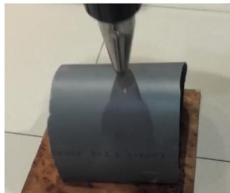
*Using a heat gun to bend and shape a plastic*
