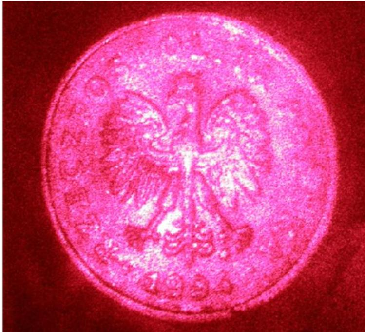
*Fig. 6 Hologram of coin recorded in the experiment*
